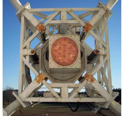
*Figure 7. 19-element phased array feed mounted on Green Bank 20-Meter Telescope (Jeffs, et. al 2008)*
